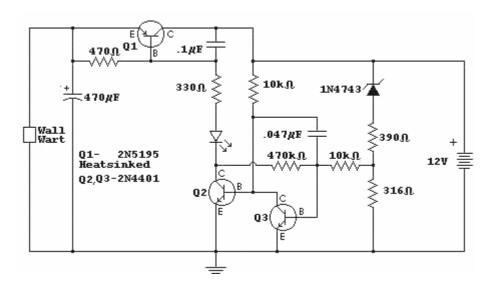
Here is an experimental (and simple!) regulator for alternator chargers.
